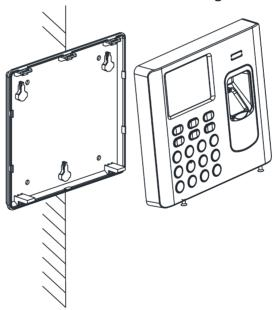
**Figure 3-5 Install Front Cover**
