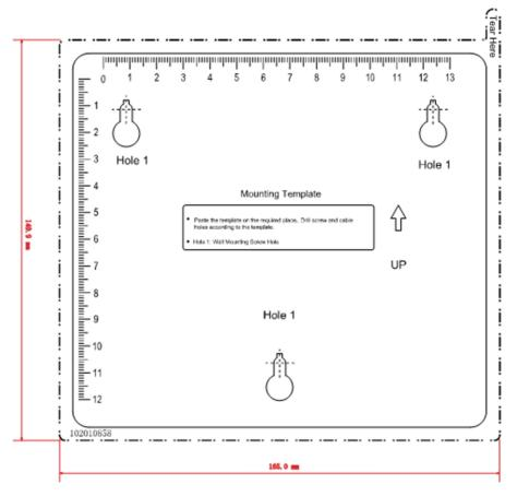
Figure 3-1 Mounting Template
